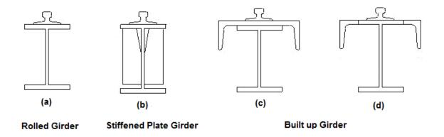
In some cases reinforcement or capping may be necessary to give resistance to lateral forces. This capping, usually channels, figure (c) or angles, figure (d), increases the lateral stiffness as well as the moments of inertia and the section moduli in compression. Capping should be used only in special instances where a wide flange beam does not quite meet the requirements of the width of flange or compression, or a welded girder should be less economical.
