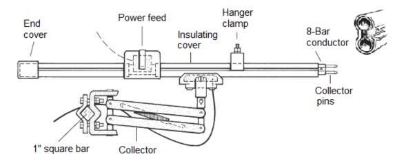
Power supply to the runway electrification consist of a series of insulated bars made out of galvanized steel, copper, stainless steel, or aluminum, which transmit electricity through sliding collector assemblies that power the motors, trolleys, hoists, etc.
