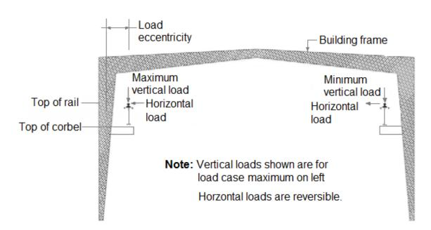
The crane runway girder is usually designed as a simple span beam and the structural analysis of the beam involves determining the location of the maximum design moments and shear due to the crane traveling along the length of the crane beam. When performing the analysis, both the horizontal forces (lateral and longitudinal) are assumed NOT to act together with the vertical loads simultaneously. Only one of them is considered to be acting with the vertical load at a time.
