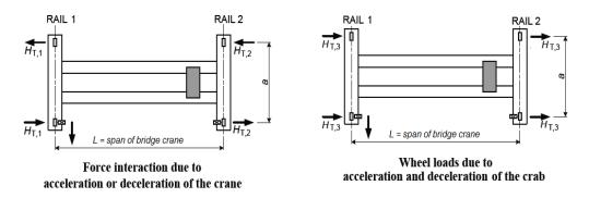
$H_{T1}$  and  $H_{T2}$  are the horizontal lateral or transverse forces at the wheels, which act as a couple as a result of the force moment.  $H_{T1}$  and  $H_{T2}$  are influenced by the wheel spacing (a) and the dynamic behavior of the crane during acceleration and deceleration. Provided that the payload is free to swing, the horizontal load  $H_{T3}$  represents the horizontal transverse wheel force related to the movement of the crab. The wheel forces can also be in an opposite direction.
