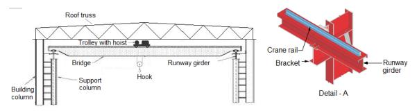
Crane runways should be thought as a stationary part of the building structure and are designed accordingly.
