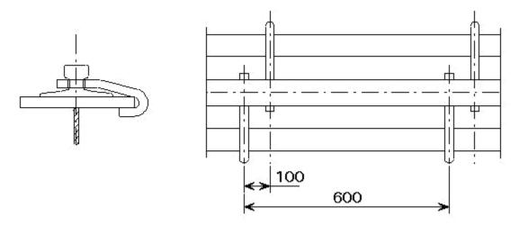
RAIL FASTENINGS USING HOOK BOLTS
